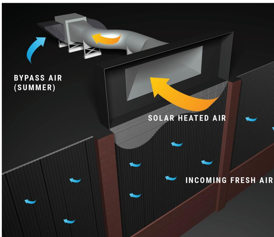
**Make-up air preheating system diagram from ATAS International. The collector is located upstream of the air handling unit to directly preheat incoming outside air. This type of system is often found in schools and institutional buildings. It is also perfect for spray paint booths, driers, and 100% outside air systems.**
